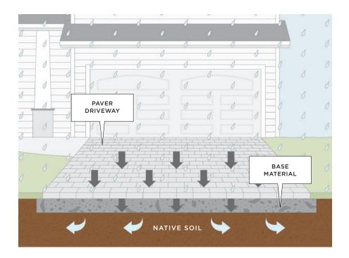
**INTERESTING FACT** A permeable paver will accumulate less ice because water will drain from the paver surface before it has time to freeze.
