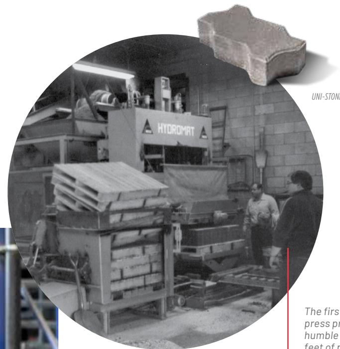
The first Unilock press produced a humble 817 square feet of pavers a day.
