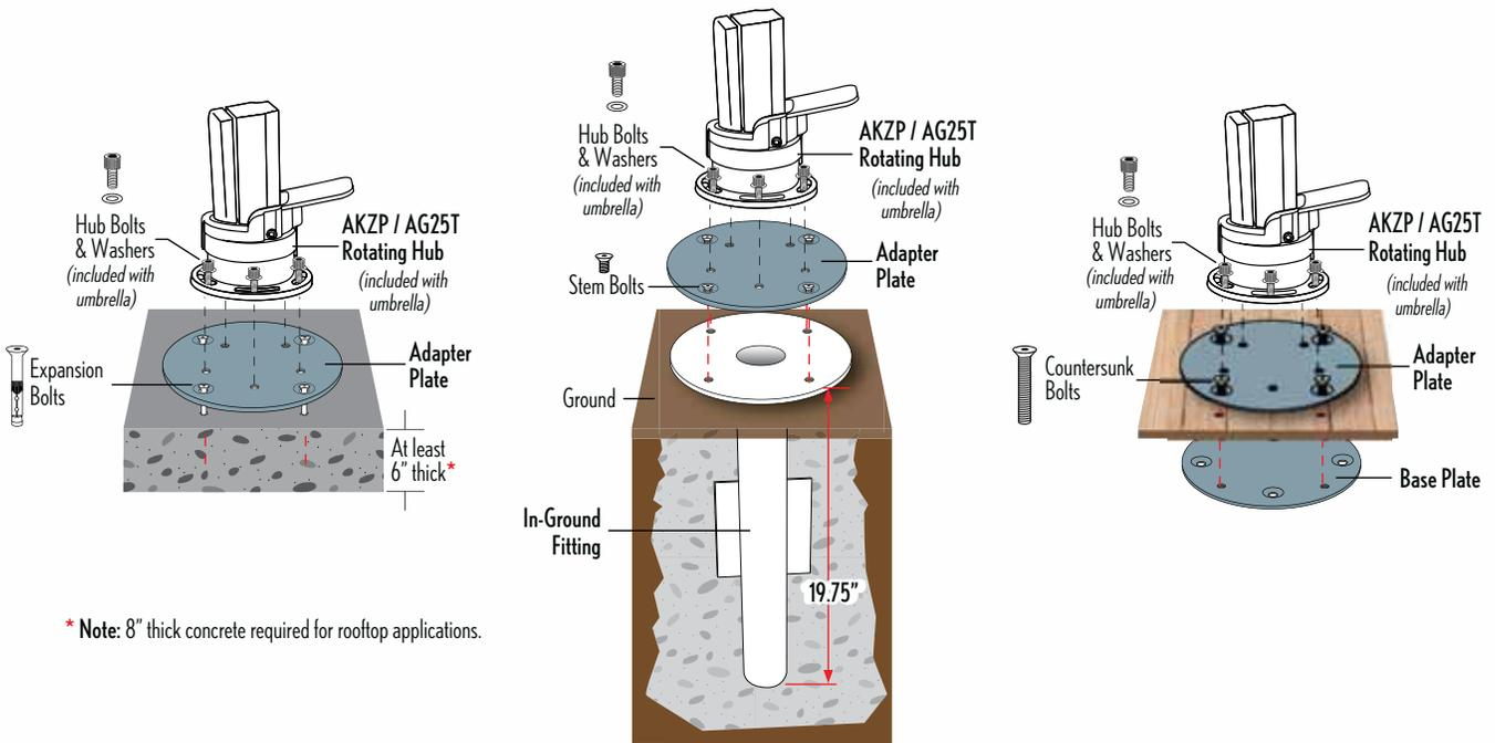
\* Note: 8" thick concrete required for rooftop applications.
