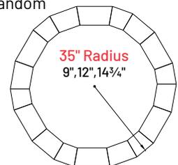
Although the three tapered unit sizes come packaged together, they can be separated to achieve various radius projects. If you construct a radius using only one size unit, the other units will be left over. Careful planning will allow you to use these units elsewhere.
