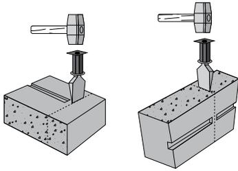
To split a large convertible unit, use a hammer and chisel to score the top and sides, then flip the unit upside down and use the chisel to break the unit. This may require a couple of hits along the groove to achieve a clean break.
