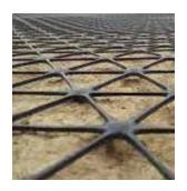
Unilock DriveGrid Geogrid is an advanced product specifically designed for trafficked surfaces. DriveGrid Geogrid's multi-directional properties leverage triangular geometry, one of construction's most stable and widely utilized shapes, to provide an enhanced level of in-plane stiffness. Its triangular structure, coupled with improved rib and junction geometry, offers the construction industry an improved alternative to conventional materials and practices.
