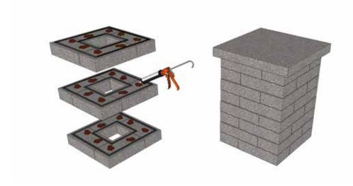
Lineo is not a retaining wall. Lineo is a decorative landscape wall, with a typical height of 12" - 16" above grade. (Higher walls are possible when engineered by a professional engineer.)
