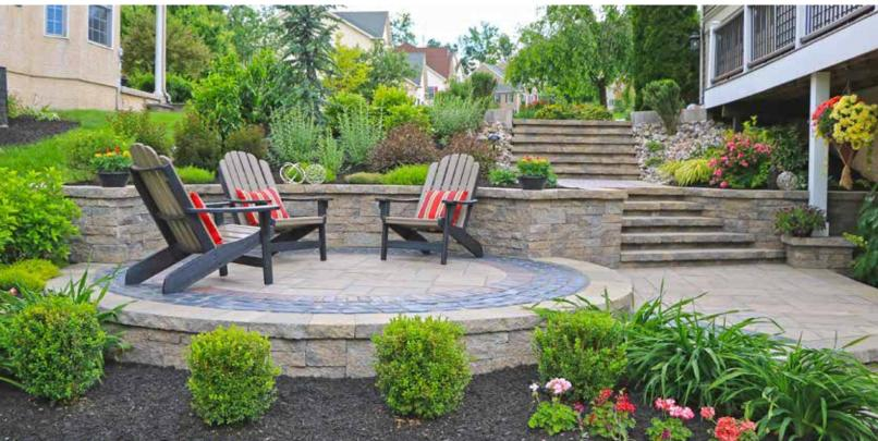
The enhanced Estate Wall System with 3" high and 6" high units, is ideal for all residential landscape walls and vertical element construction. The front and back of each unit is rock-faced making it perfect for seat walls and the unique tapered units can be used for both straight or curved applications.
