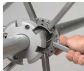
HUB The hub is cast aluminum and engineered for extra strength. It is split horizontally to encapsulate the stainless steel direct connect pin assembly. Two screws secure the hub together.
